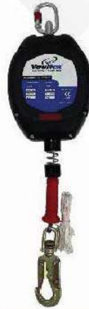
REF NO: PMS ORIGINAL BRAND: VAULTEX RETRACTABLE FALL ARRESTER - 15 METER 4.8 MM STEEL ROPE CAPACITY: 100 KG EN 360:2002 CE 0082
