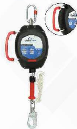
REF NO: TRA ORIGINAL BRAND: VAULTEX RETRACTABLE FALL ARRESTER - 12 METER 4.8 MM STEEL ROPE CAPACITY: 100 KG EN 360:2002
